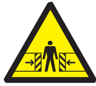
Danger of entrapment
